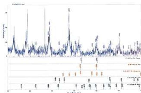
Fig. 1 XRD diffractogram of the Popa manganese ore sample
