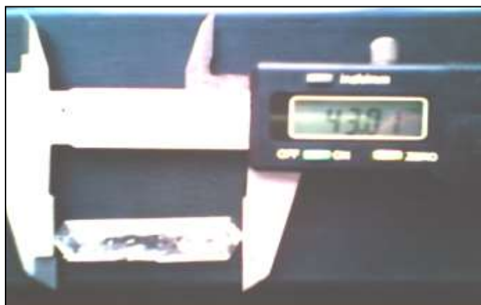
Fig. 1 Photograph showing the as-grown crystal of \text{Li}^{3+} (1 mol%) doped \text{MgSO}_4 \cdot 7\text{H}_2\text{O}
