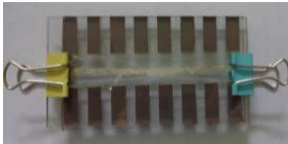
Fig. (7) Assembling a series and parallel connected DSSC module
